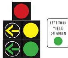
This five light signal arrangement is commonly used. It allows for “protected” left turns, when the green arrow is displayed that
