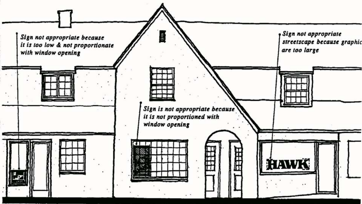
WINDOW SIGNAGE NOT APPROPRIATE
